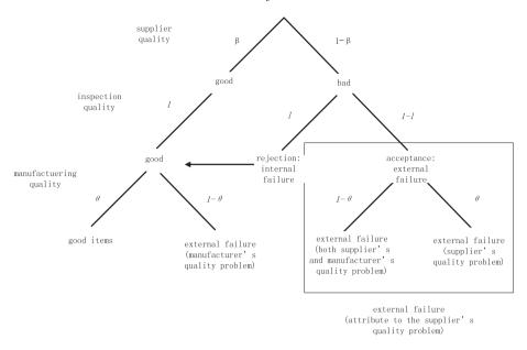
Figure 1. A probability tree of external failure.
